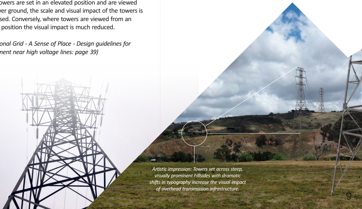
Flat or slight to moderate undulating open topography, well away from neighbours and towns reduces visual impact and represents a more acceptable option when siting overhead transmission infrastructure.
